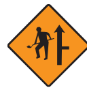
Site access on right
