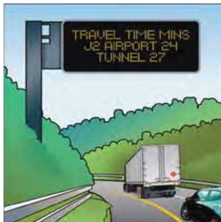
Typical LED VMS
